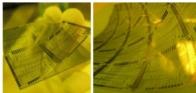
Example test cell device on plastic in a top gate configuration. Lithographically defined electrodes to 5µm channel length resolution
